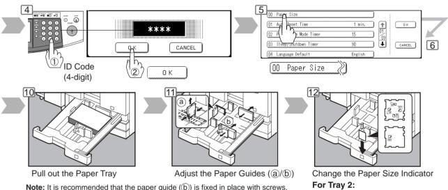
**Note:** It is recommended that the paper guide ((b)) is fixed in place with screws. Consult an authorized service provider for details on how to fasten the guide.
